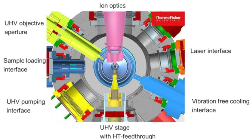
**Figure 2:** Schematic outline of the arrangement of the main components in the objective lens octagon.
