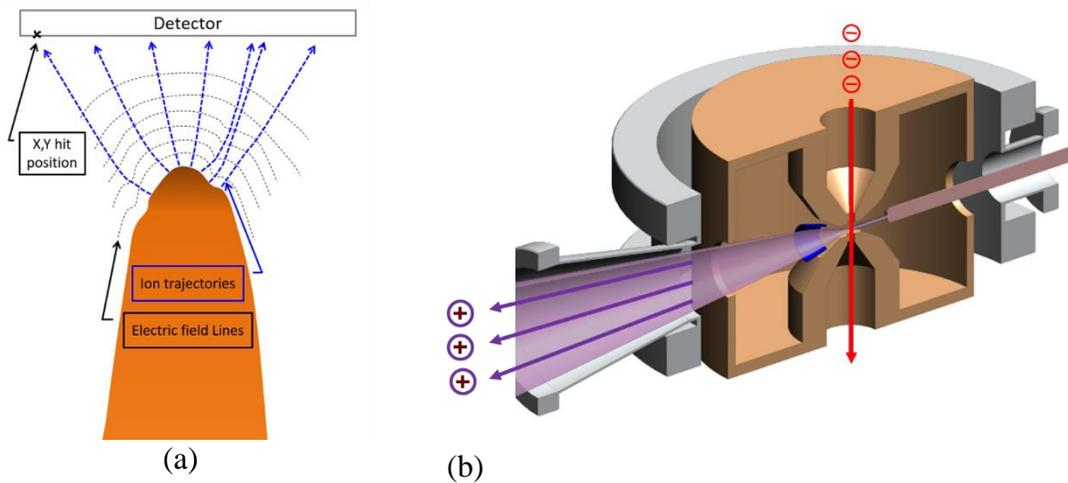
**Figure 1:** (a) Effect of the apex shape on the APT results of a multiphase sample: schematic drawing of how the electric field line geometry influences the ion trajectories and registration positions on the two-dimensional detector. (b) Schematic drawing of the integration of the APT needle in the centre of the pole piece lens of the TOMO-TEM. UHV conditions and temperatures below 35 K will be ensured by a completely new column and stage design.
